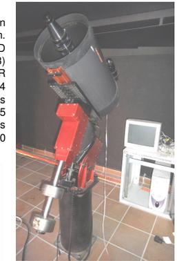
Figure 1. Watec 902H Ultimate CCD video camera and one of the SC telescopes (0.36 m) employed to record the impact flash presented here.
